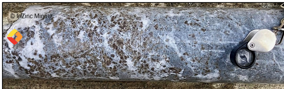
Hole IB26-051 HQ core at 77.6m: Coarse crystals of sphalerite (brown - up to 1 cm) in a quartz-carbonate-barite stockwork. Representative photo of interval from 72.1 to 82.1 m (10.0 m grading 7.4% Zn, 1.3% Pb and 7.7 g/t Ag).
