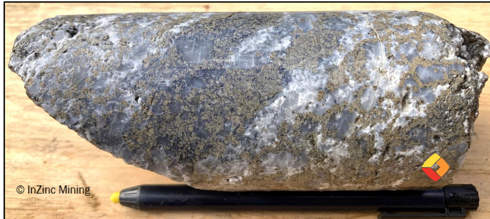
Replacement style mineralization - dominantly sphalerite (light brown-tan) and minor pyrite from Hole IB25-043 (HQ core size, marker crayon for scale at base). This core section is included in a sample totalling 0.7 m in length (from 200.00 m to 200.70 m downhole) grading 27.4% Zn, 1.8% Pb and 10.2 g/t Ag with 5.63 ppm gallium (sample 376827).
