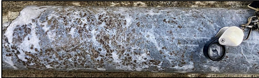
Figure 2: Drill Hole IB26-051 – Coarse Crystalline Sphalerite (Zinc)
